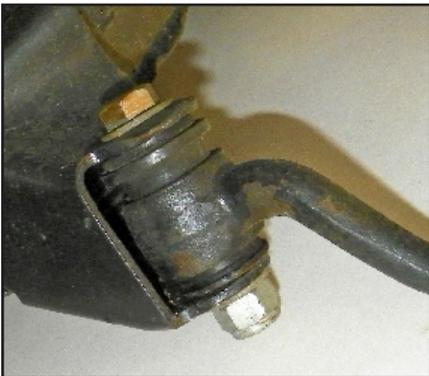
By 1968, Ma Mopar had seen the light, and gone to this double-shear design. Still, the internal rubber bushings lack precision.
