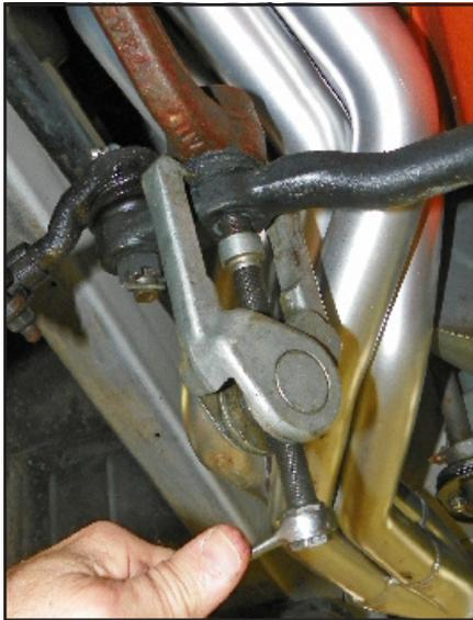
Installation is easy but differs a bit from stock. Remove the old idler; always use a puller on tapered joints.
