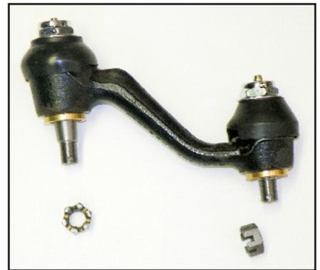
Firm Feel ([www.firmfeel.com](http://www.firmfeel.com)) has come to our rescue, with their Torrington-needle-bearing equipped idler. It is not only greaseable, but adjustable. Even 50 years from now, simply snugging the adjuster nuts will reduce slop to zero.
